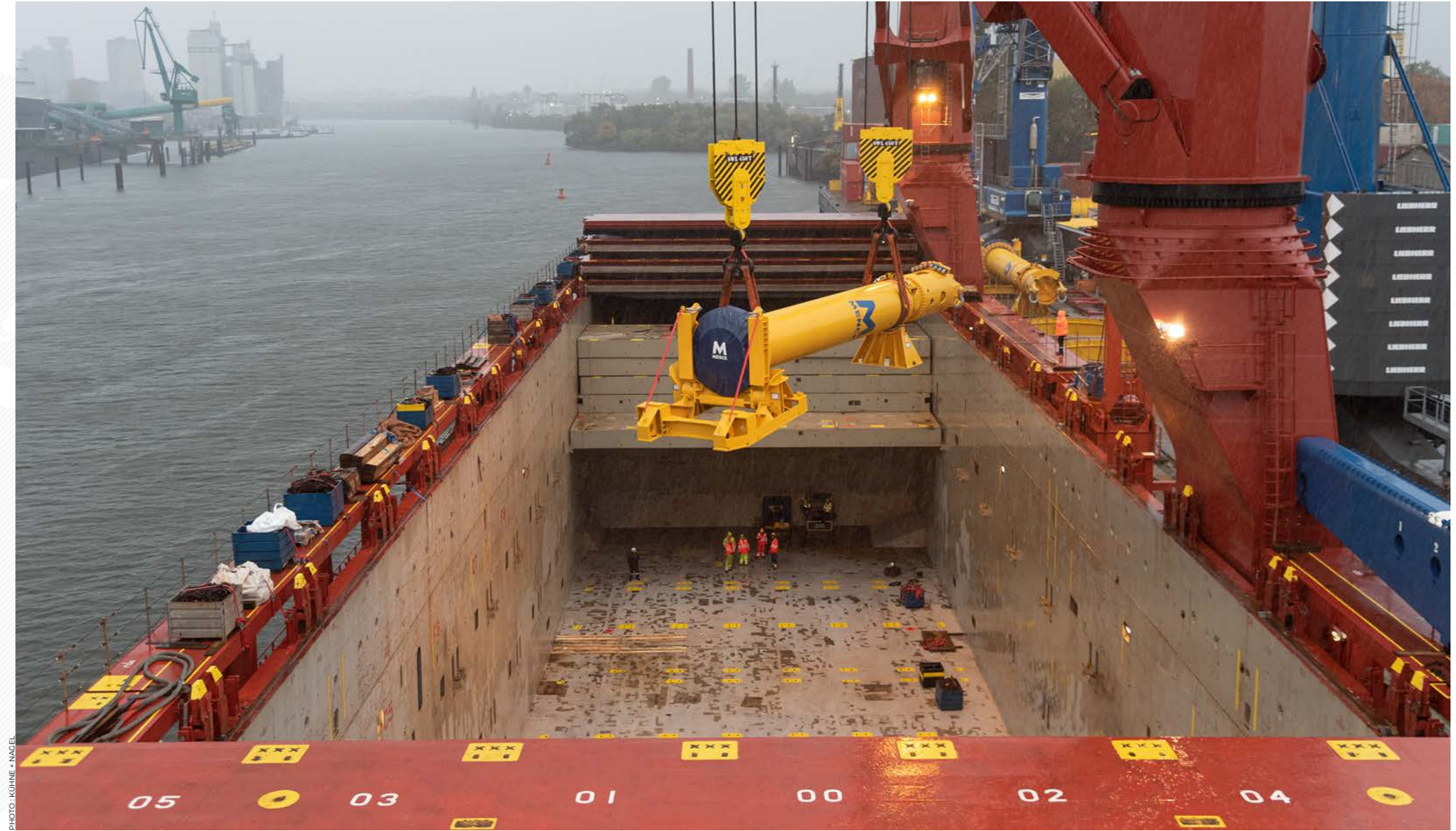
F900 Eco-Lifter MV UHL Focus loads an offshore hydraulic hammer weighing 300 mtons in the port of Hamburg (Germany).
