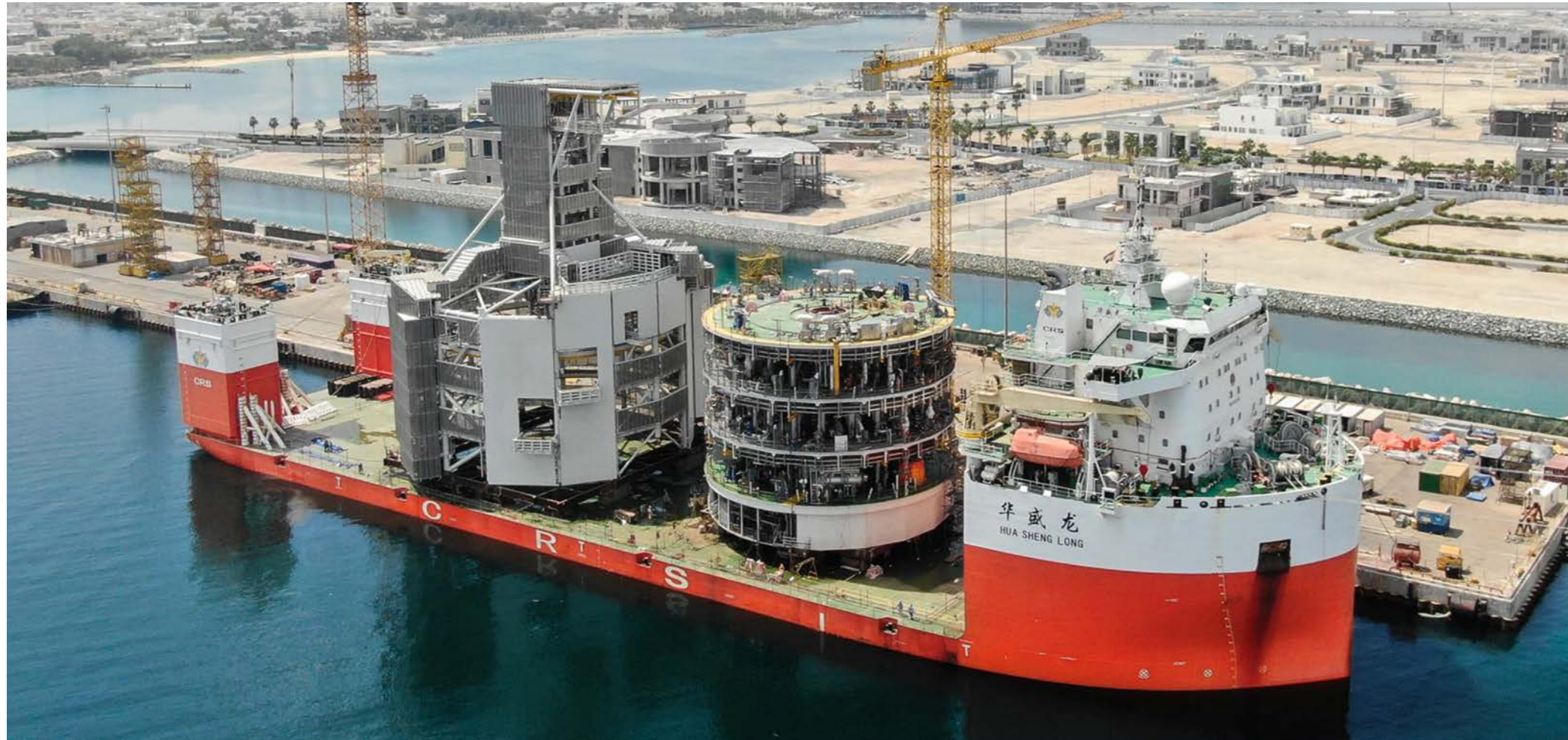
Above project: Johan Castberg FPSO – Turret mooring system transport in 2019 - 2020 | Scope of work: Ocean transport of 8,000 mtons turret from Dubai (UAE) to Singapore | Utilizing two semi-submersible heavy transport vessels and one heavy lift vessel to transport all modules | In-house project management | Engineering, design, and fabrication of the transport grillage/cradles and all seafastening of the cargo
